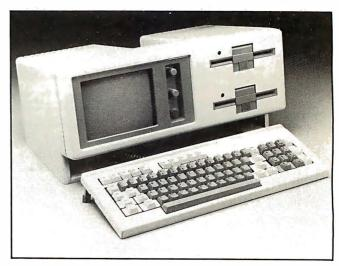
The ultra-light 20-lb. Hyperion features a 7-in. amber screen and 5.25-in. double-sided double-density drives. The shift key is placed more strategically than on the IBM PC.
