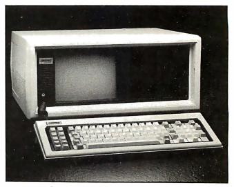
The 28-lb. Compaq has a 9-in. display and a keyboard remarkably close to the IBM's.
