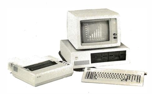
The system as tested costs \$4,550 and includes 64K bytes of user memory, two minifloppy disk drives holding a total of 320K, keyboard, green-tint monochrome display, and the modified Epson MX-80 printer that is sold under the IBM label. The IBM DOS operating system was used; standard software includes Basic (located in permanent read-only memory), file handling utilities and a screen-based program editor.
