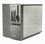
users. The Spirit is targeted to professional, legal and financial services firms with requirements for powerful, reliable, growth-oriented computing. The product line combines functionally dense single-board computer (SBC) architecture in conjunction with the new VME bus, a joint standard of Motorola, Philips/Signetics and Mostek corporations. The high-speed VME bus makes possible the combination of
