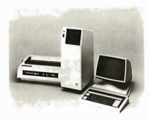
a 10-by-14 grid (80 column-by-24 lines) with a choice of three display colors. Voyager's monitor adjusts up/down and rotates 359 degrees. Its detachable keyboard has 100 five function definable keys and a 10-key calculation pad. Voyager Systems, Newbury Park, CA.
