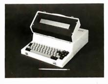
system includes 64K bytes of main memory for computation and 4K bytes of memory for communications. A full-size, high-quality keyboard and a four line-by-80 character display make the 15-pound computer easy to use. A full 24 lines-by-80 characters of information are held in memory. This allows the four-line display to act as a window to look at any desired area at will. A 5.25-in. floppy disk drive and power supply/recharger are included. The floppy disk
